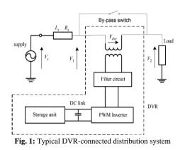
The major custom electrical devices which are used in distribution system for power quality improvement are Distribution STATIC synchronous compensator (DSTATCOM), Dynamic Voltage Restorer (DVR), Active Filter (AF), Unified Power Quality Conditioner (UPQC) etc. From the above custom energy devices, right here DVR is used for the power exceptional improvement in the distribution system.
