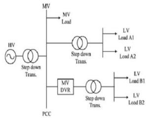
Fig. 3: DVR join in a medium-voltage level electricity systems
