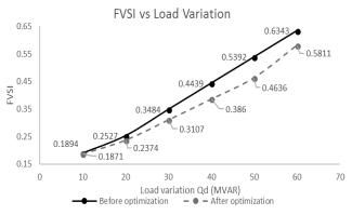
Fig. 3: Comparison of FVSI before and after optimization.
