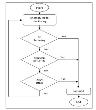
Fig 1: Process Flow for detecting jamming attack in MAC and physical layer.
