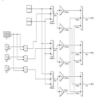
Fig. 6: Three-phase inverter based on the relation of induction motor phase voltages and pole voltages
