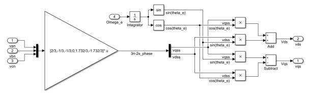
Fig. 3: Simulink implementation of equation (1), (2) and (3)
