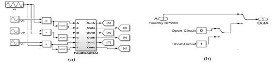
Fig. 8: (a) Modified SPWM generator (b) SPWM signal bypass
