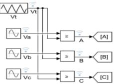
Fig. 5: Simulink implementation of SPWM switching signal generator
