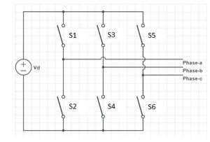
Fig. 4: Typical three-phase inverter topology
