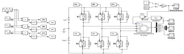
Fig. 7: Complete model of the three-phase induction motor drive in Simulink
