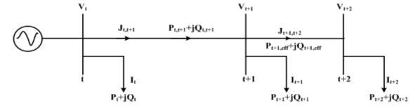
Fig. 1: Simple distribution system
