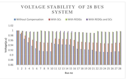
Fig. 4: Voltage stability of 28-bus Indian distribution network
