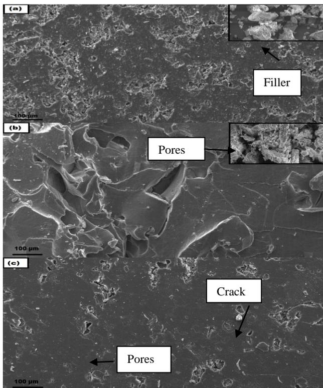
**Fig.6:** SEM images of silicone rubber modified by (a) wollastonite (5 wt.%) (b) silica (10 wt.%) (c) pure SiR after the tensile test (enclosed particles of wollastonite and silica at each micrographs).
