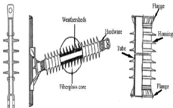
Fig. 1: Designs and types of composite insulator (14)
