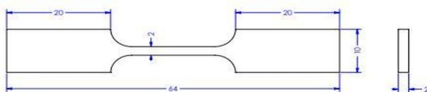
Fig.2: Sample for mechanical tensile testing
