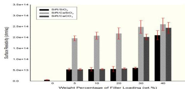
Fig. 5: Results for electrical surface resistivity testing
