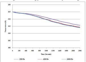
Fig. 8: The fall of temperature with respect to flow velocities while cooling
