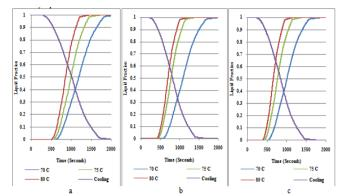
Fig. 4: Liquid fraction with respect to time at inlet temperatures at flow of a) At  $R_e = 2000$  b) at  $R_e = 4000$  c)  $R_e = 10000$
