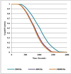
Fig. 6: Liquid fraction Vs Flows velocities (cooling)
