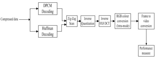
Fig. 1: Block diagram of the HSV-EPHC-IFHEVC system
