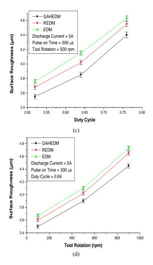
Fig. 5: Influence of (a) discharge current (b) pulse on time (c) duty cycle (d) tool rotation on SR
