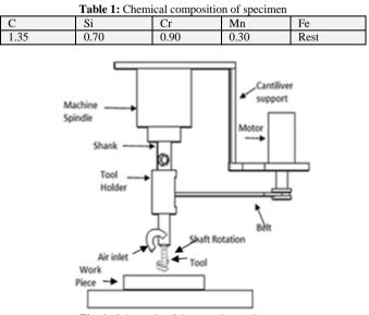
Fig. 1: Schematic of the experimental setup.
