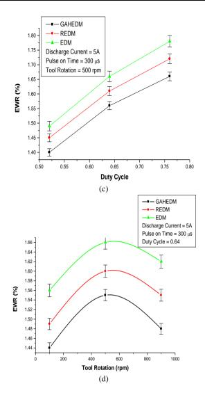
**Fig. 4:** Influence of (a) discharge current (b) pulse on time (c) duty cycle (d) tool rotation on EWR
