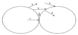
Fig. 4: Heat transfer paths between particles (Yagi & Kunii, 1957).
