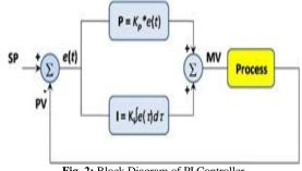
Fig. 2: Block Diagram of PI Controller
