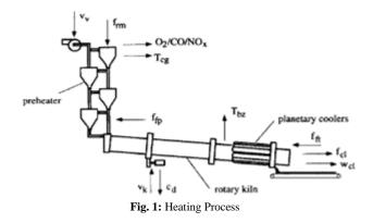
Crude supper must be preheated and totally gone away before it is bolstered into the oven. Hot smokes created in the oven amid the clinker generation are utilized. Pre-radiator is mindful to secure the remained damp- ness of the crude material and separate silicates, and also calcinate mostly the present carbonates in the ma- terial.
