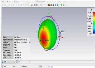
Fig. 4: Gain of presented design at 1.42GHz
