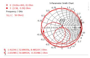
Fig. 3: Analysis of impedance matching of presented design
