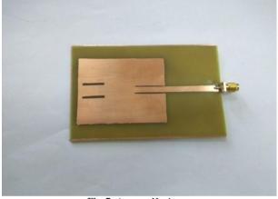
Fig. 7: Antenna Hardware
