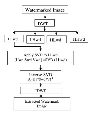
Fig. 3: Watermark extraction block diagram
