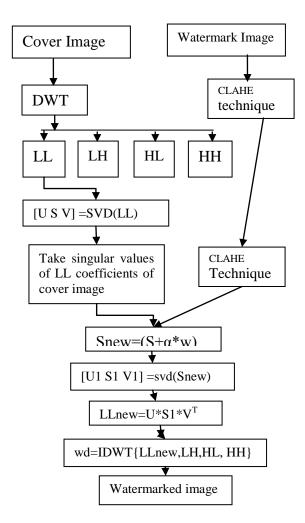
Fig. 2: Watermark embedding block diagram
