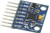
Fig. 3: MPU6050 Accelerometer & Gyroscope Sensor
