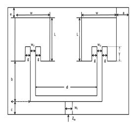
Fig. 3: Corporate fed microstrip patch antenna array
