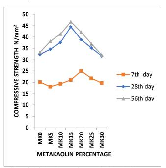
Figure 1 Variation of compressive strength with metakaolin content
