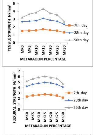
Figure 2 Variation of Tensile strength and flexural strength with metakaolin content
