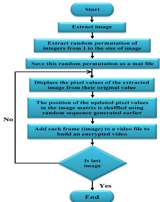
Fig. 7: Flow Chart for Encryption.
