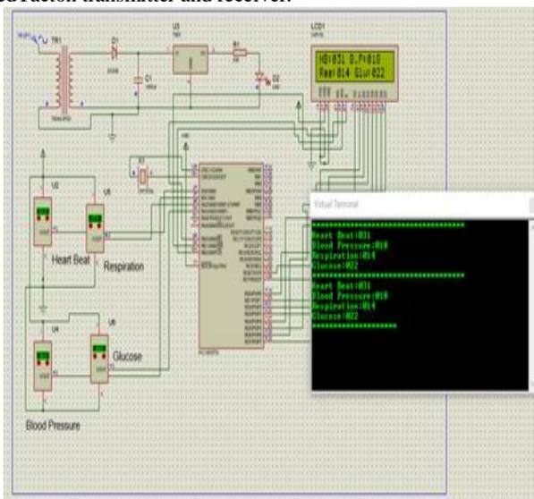
Fig. 3: Simulation result of biotelemetry system
