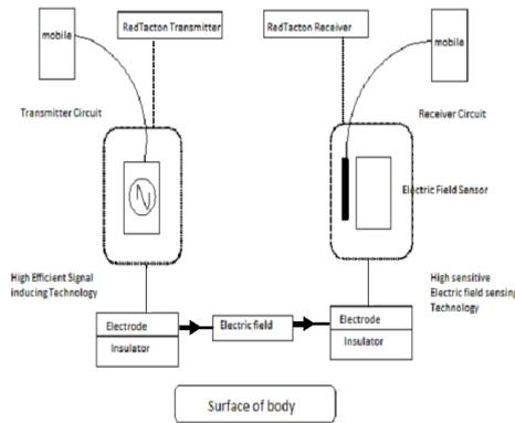
Fig. 2: Working principle of RedTaction technology
