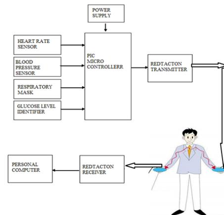
Fig. 1: Biotelemetry system
