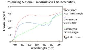
Figure4:. Transmittances of polarizing film
