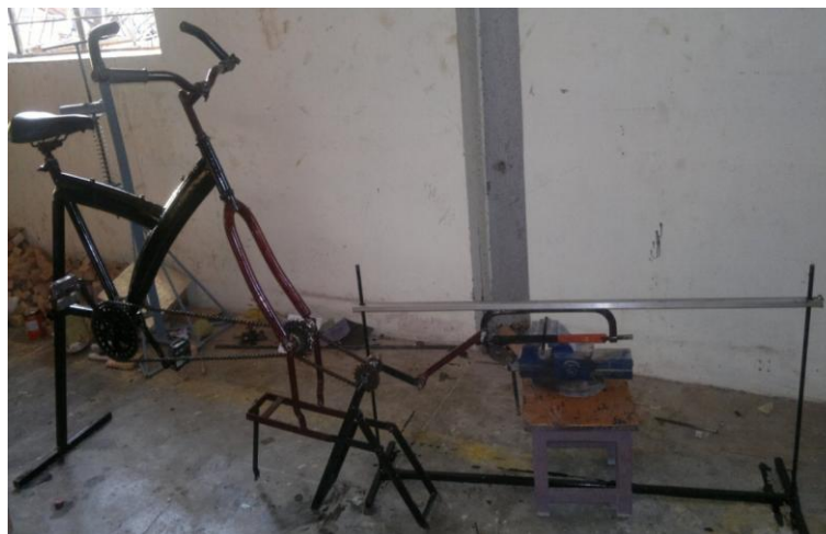
Fig. 4: Working Model - Dual chain drive Hacksaw Cutter
