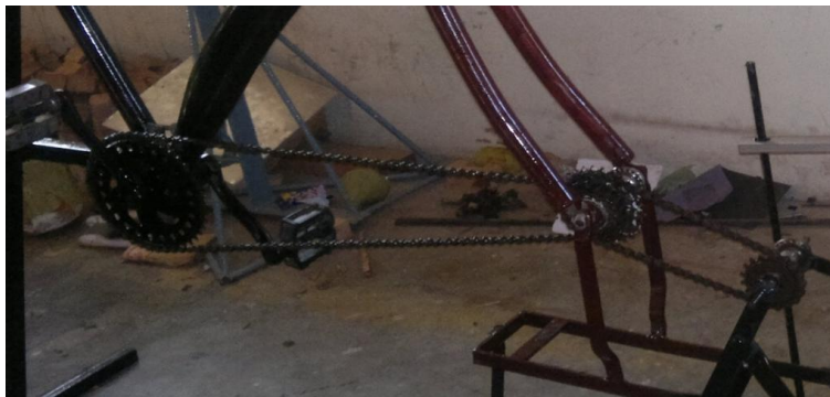
Fig. 2: Dual Chain drive
