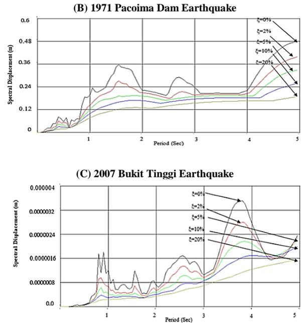
Fig. 4: Graphs of Spectral Displacement Earthquake Versus Time.
