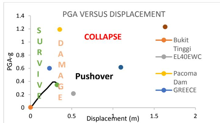
Fig. 7: Level of Safety Under Seven Past Earthquake Records.
