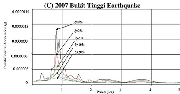
Fig. 5: Graphs of Pseudo Spectral Acceleration Versus Time.
