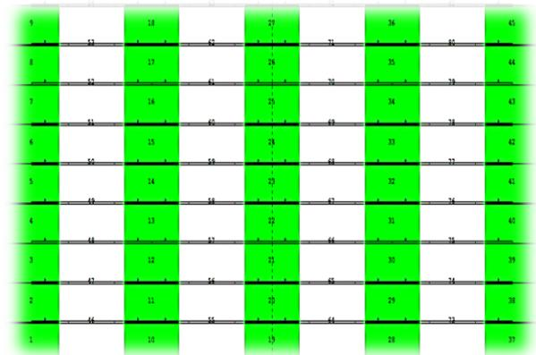
Fig. 2: Number of Nodes and Elements for Four Bay Nine-Story Tunnel Form Building Using Ruaumoko 2D Program.
