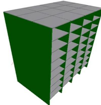
Fig. 1: Isometric View of Four Bay Nine-Story Tunnel Form Building Using STAAD PRO Program.
