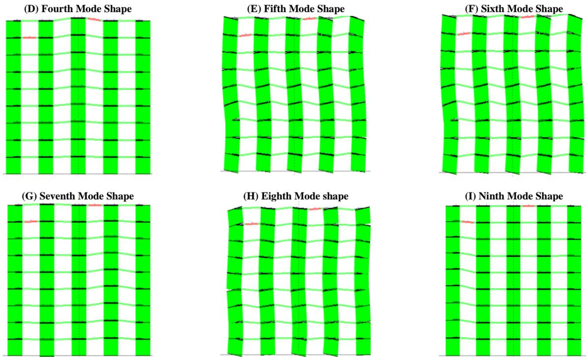
Fig. 6: Nine Mode Shape for Nine-Story Tunnel Form Building Under Seven Earthquake Excitations.
