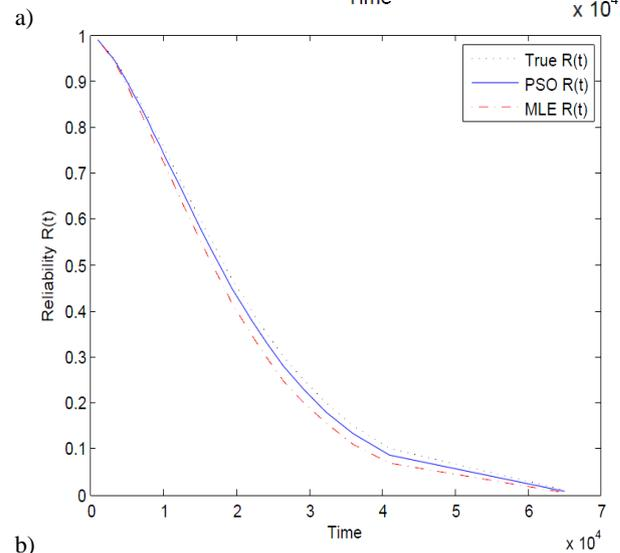
Fig. 2: Plot of probability density function (a) and reliability (b) against time
