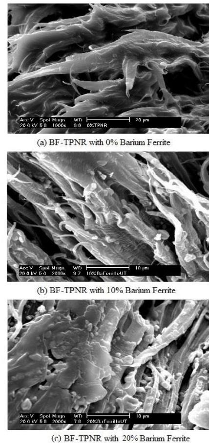
**Fig. 2:** Scanning electron micrographs (SEM) of the microwave absorber composite. (a) 0% BF, (b) 10% BF and (c) 20% BF.
