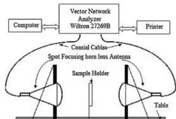
(c) schematic diagram of microwave NDT system
