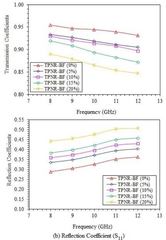
Fig. 5: Scattering parameters (reflection and transmission coefficient) of TPNR-BF.
