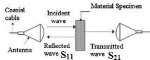
(b) Incident, reflected and transmitted wave
