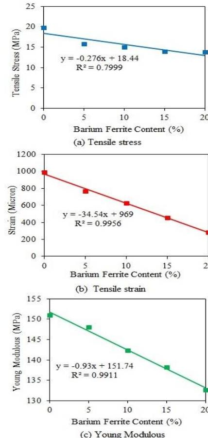
**Fig. 3:** The mechanical properties of the TPNR-BF at different filler content. (a) tensile stress, (b) tensile strain, and (c) Young modulus.
