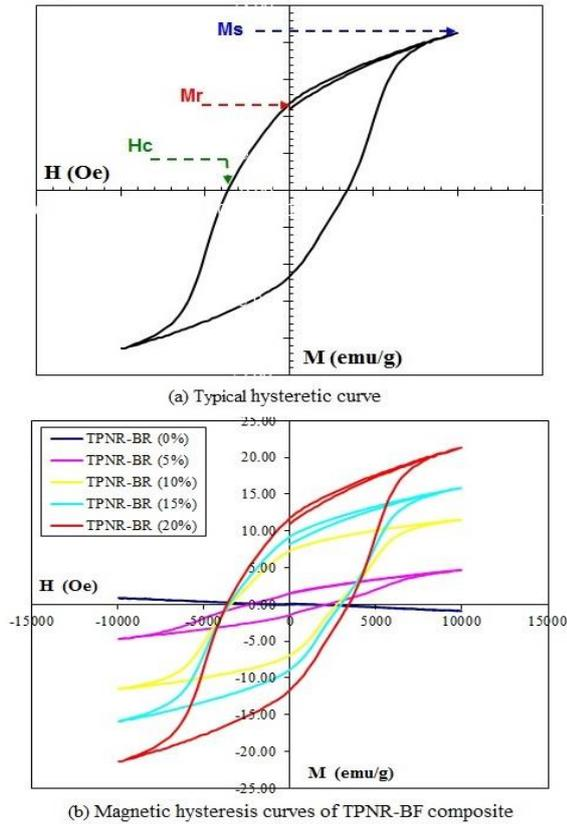
Fig. 4: Magnetic properties (H vs M curve) of TPNR-BF composite.
