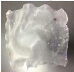
Fig. 13: A sample of bioplastic after ten (10) days undergo water absorption test
