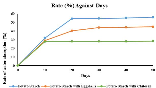
Fig. 12: Rate of water absorption (%) against days for water adsorption test
