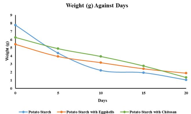
Fig. 14: Weight (g) against days for biodegradability behaviour test
