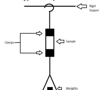
Fig. 4: Illustration of Tensile Test on the bioplastic
