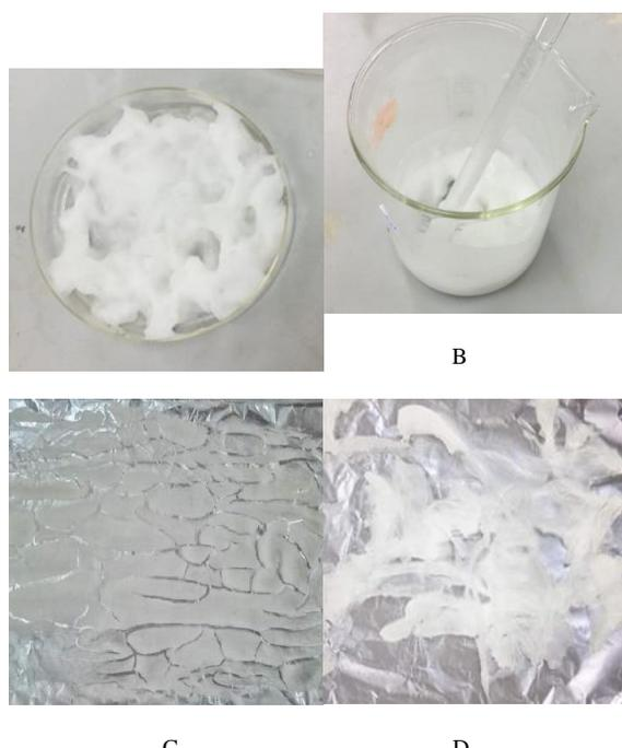
Fig. 7: A) 1<sup>st</sup> trial – Wet condition, B) 3<sup>rd</sup> trial – Early hardening, C) 2<sup>nd</sup> trial – Cracking before its rigid state, D) 2<sup>nd</sup> trial – Cracking after its rigid state
