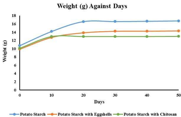
Fig. 11: Weight (g) against days for water adsorption test
