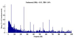
Fig. 5: Total Harmonic Distortion of Load Voltage.
