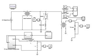
Fig. 1: Simulation Block Diagram of Single Phase DVR.
