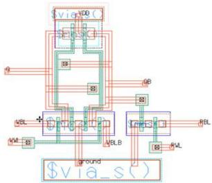
Fig. 10: Layout for Conventional 8T SRAM Cell.
