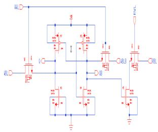
Fig. 3: Proposed 8T SRAM with Read Assist.
