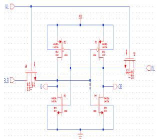
Fig. 1: Standard 6T SRAM Cell.
