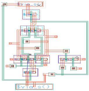
Fig. 12: Layout for 8T SRAM Using Two Extra Pass Transistors.
