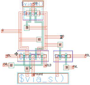
Fig. 11: Layout for Proposed 8T SRAM with Read Assist.
