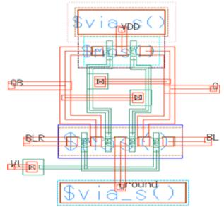
Fig. 9: Layout for Standard 6T SRAM Cell.
