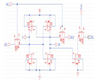
Fig. 2: Conventional 8T SRAM Cell.
