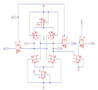
Fig. 4: Proposed 8T SRAM Using [2] Extra Pass Transistors.
