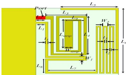
Figure 2.: Radiating Element Structure
