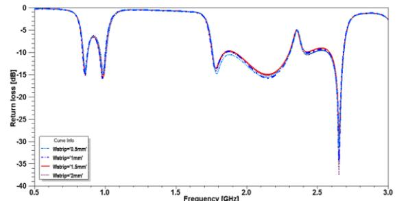
Figure 10: Parametric investigation on varying the length of the strip 'Wstrip'
