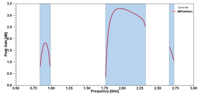
Figure 8: Peak Gain Vs Frequency characteristics
