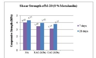
Fig. 5: At 7-Days & 28-Days Shear Strength of Selected RAC and CAC without Metakaolin for M-20.
