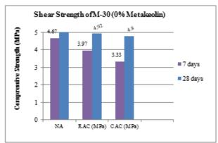
Fig. 6: At 7-Days & 28-Days, Shear Strength of Selected RAC and CAC without Metakaolin for M30.
