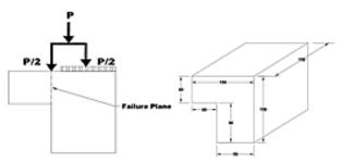
Fig. 3: Dimensions of Specimen and Loading Setup.
