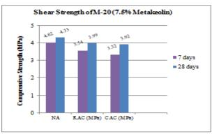
Fig. 8: Shear Strength of Selected RAC and CAC with 7.5% Metakaolin for M-20.
