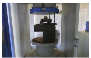
Fig. 4: Experimental Set Up for Shear Test.
