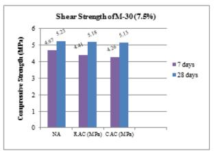
Fig. 11: Shear Strength of Selected RAC and CAC with 7.5% Met kaolin for M30.
