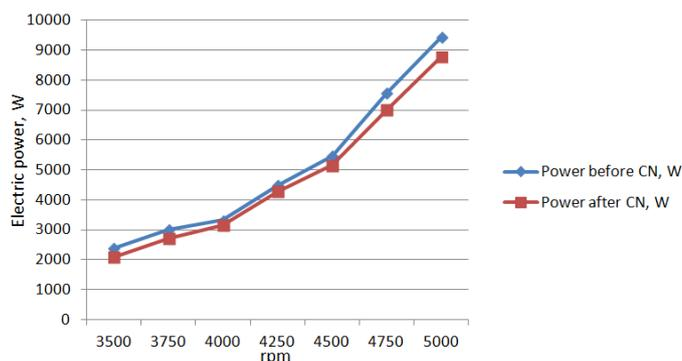
**Figure 1:** Electric power of the turbogenerator before and after the catalyst neutralizer.
