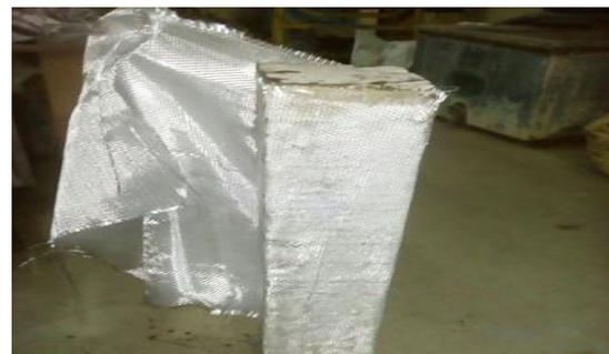
Fig.3: Wrapping of GFRP
