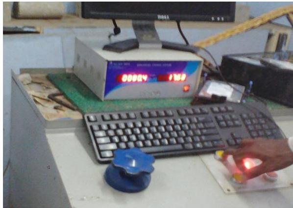
**Fig 5:** Digital Deflectometer
