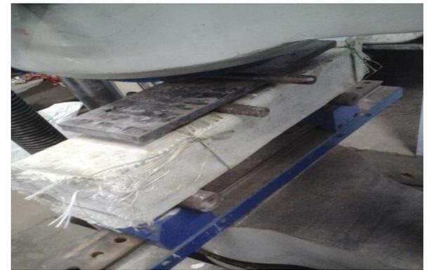
**Fig.8:** Testing of UDDL beam specimen
