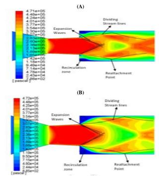
Fig. 3: Close View of CD Nozzle with Pressure Flow (A) with Control (B) Without Control.
