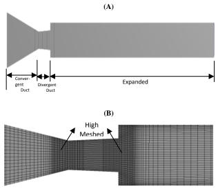
Fig. 2: 2D Planar Fluid Body (A) Finite Element Model (B) Meshing.
