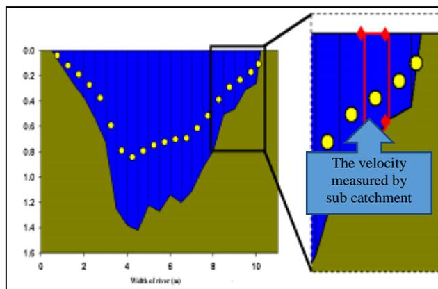
**Fig. 5:** Discharge measurement by cross section of the river [10]
