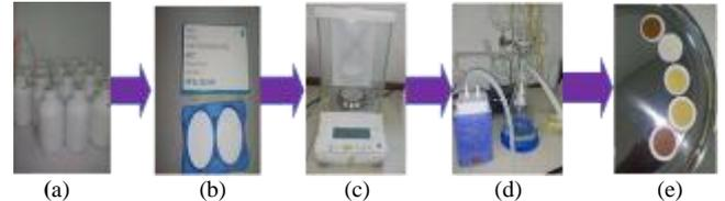
**Fig. 2:** a) Sample water b) Membrane filter c) Electronic weighing d) Filtration apparatus with vacuum pump e) Dried membrane filter
