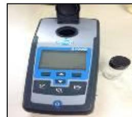
**Fig. 3:** The measurement of turbidity parameter (turbidity meter) (HACH 2100Q Portable Turbidimeter, USA)
