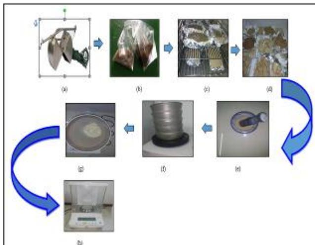
**Fig. 4:** a) Sediment Grab b) Sample Sediment c) Sediment was dried at room temperature (d) the dried sediment (e) Mortar pestle (f) Mechanical shakers (g) The sediment was sieved (h) The sediment will be weighed using the electronic weighing
