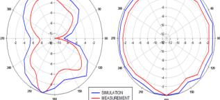
Fig. 5: Polar plot for proposed antenna (a) Phi 90 (b) Phi 0.
