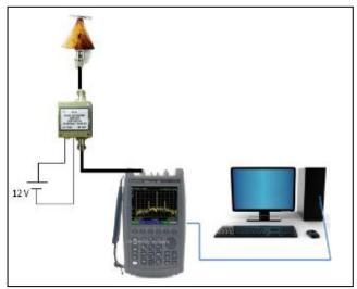
Fig. 2: The illustration of RFI connection set up [21].
