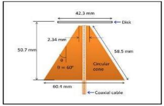
Fig. 1: The schematic geometry of the discone antenna.
