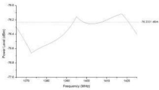
Fig. 6: Average RFI level in HI suggested minimum bandwidth
