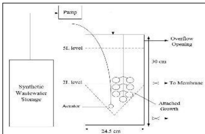
**Figure 1:** Schematic Diagram of SBR Experimental Setup.
