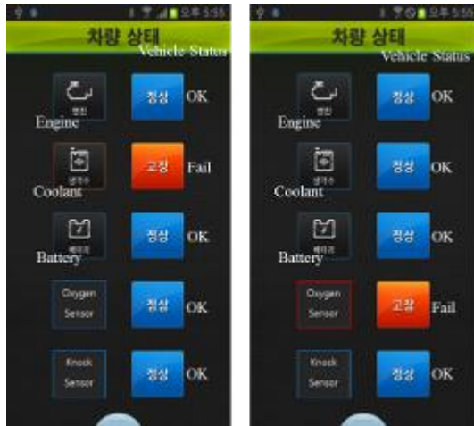
Figure 7: Fault examples in the vehicle status menu.
