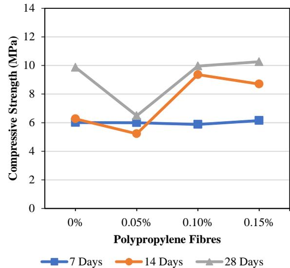
Figure 2: Compressive strength behaviour of 1600 kg/m<sup>3</sup> density of foamed concrete.
