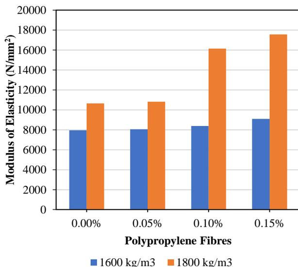
**Figure 4:** Modulus of elasticity of different densities of foamed concrete.
