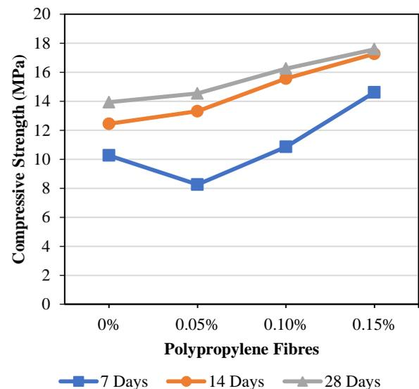
Figure 3: Compressive strength behaviour of 1800 kg/m<sup>3</sup> density of foamed concrete.
