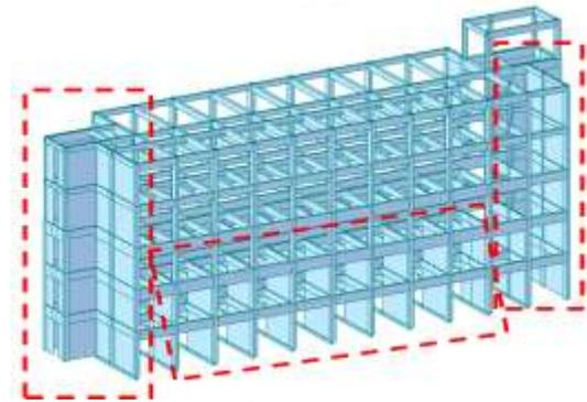
Figure 6: Structure model of the building strengthened with infilled walls
