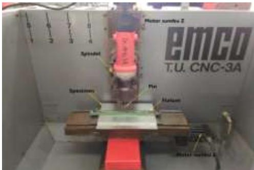
Figure 2: Equipment of  $\mu$ FSSW
