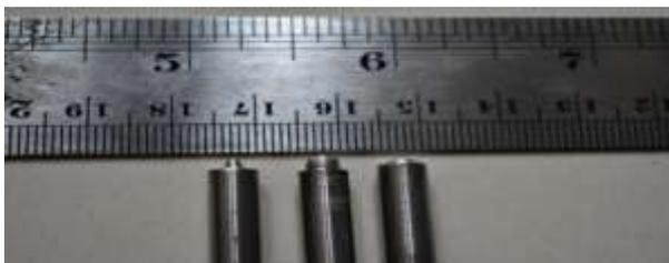
Figure 3: Weld Tool of  $\mu$ FSSW
