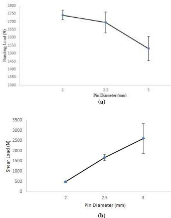
Figure 6: (a) Maximal bending load, (b) Shear load test, in variation of pin diameter
