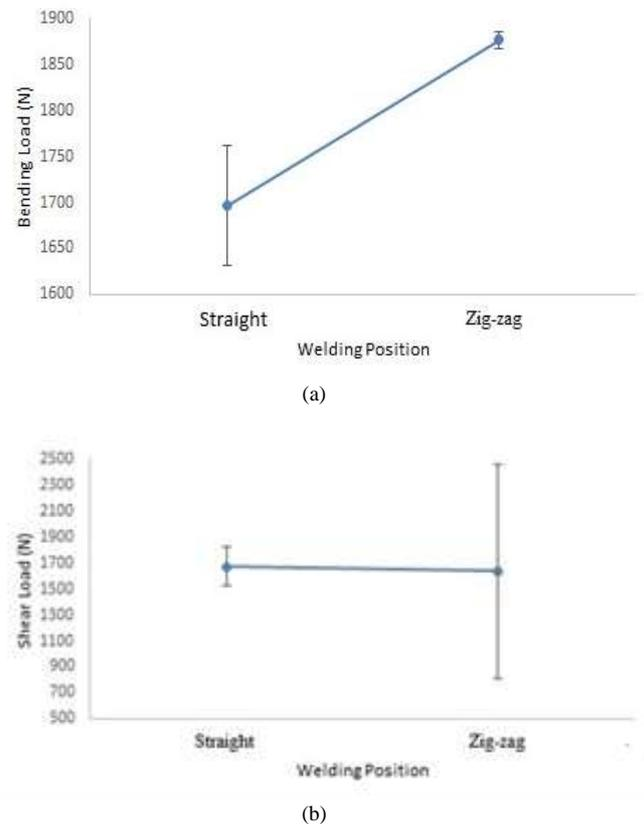
Figure 7: (a) maximal bending load, (b) shear load test in variation of welding position
