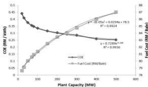
Figure 3: Relationship between plant capacity with fuel cost and COE
