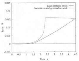
Figure 13: Exact inelastic strain curve generated by NN (Case II, Max. strain range: 0.036%)
