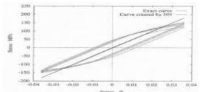
Figure 9: Exact stress-strain curve generated by NN (Max. strain range: 0.036%)
