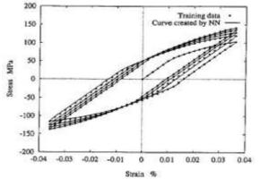
Figure 11: Stress-stain plots produced by training data and the curves produced by NN
