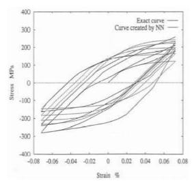
Figure 7: Exact stress-strain curve generated by NN (Max. strain range: 0.072%)
