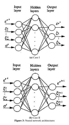
If it can describe material behavior in the form of a state space, we can apply NNs to mimic behavior and use the network as a material model. Te next section will suggest a general state space formulation of material behavior.
