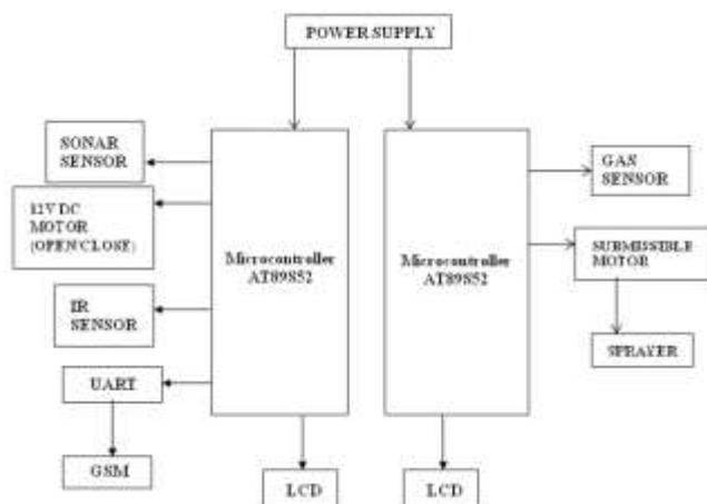
Fig 4.1: Block Diagram of Smart Dumpster Monitoring System
