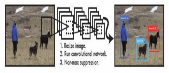
Figure 5: The YOLO Detection System
