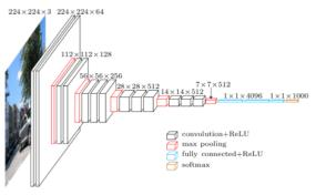
Figure 4: Architecture of VGG-16
