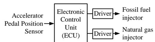
Figure 1: The ECU control for fuel injector
