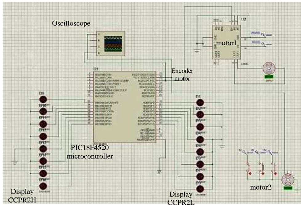
Figure 2: Schematic circuit to test functionality of the program on microcontroller.
