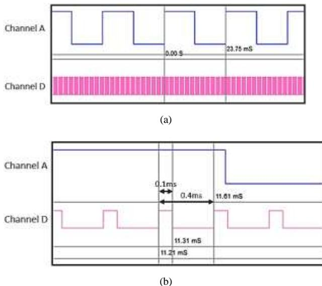
**Figure 4:** Incoming signal and generated PWM signal captured on oscilloscope; (a) Normal view; (b) Enlarge view to examine PWM signal with 25% duty-cycle.
