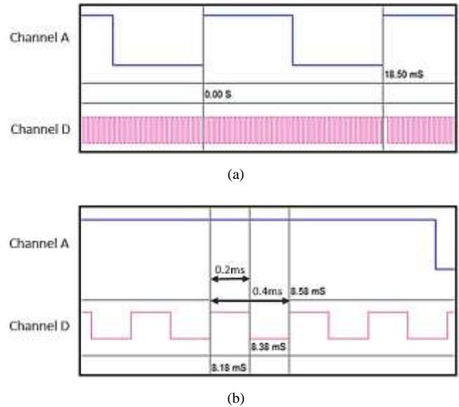
**Figure 5:** Incoming signal and generated PWM signal captured on oscilloscope; (a) Normal view; (b) Enlarge view to examine PWM signal with 50% duty-cycle.
