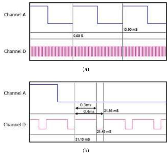
**Figure 6:** Incoming signal and generated PWM signal captured on oscilloscope; (a) Normal view; (b) Enlarge view to examine PWM signal with 75% duty-cycle.
