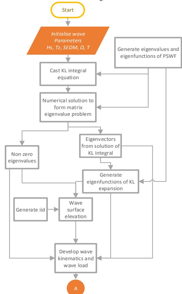
Figure 2.1: Flowchart of the algorithm for simulating wave profile
