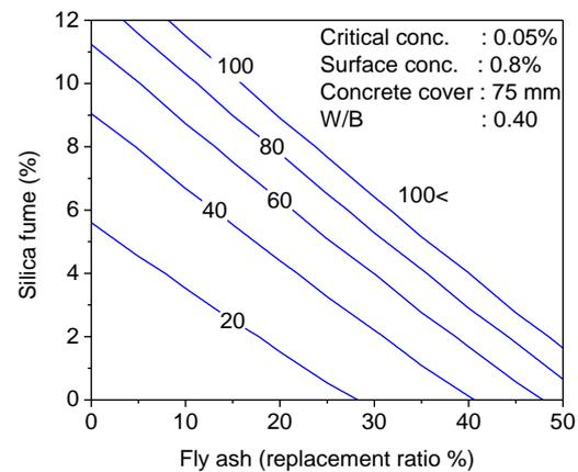
**Figure 4:** Corrosion initiation time with respect to the contents of silica fume and fly ash (W/B=0.4)
