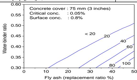
**Figure 1:** Corrosion initiation time with respect to the water-binder ratio and fly ash contents
