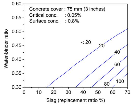
**Figure 2:** Corrosion initiation time with respect to the water-binder ratio and slag contents
