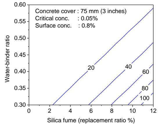
**Figure 3:** Corrosion initiation time with respect to the water-binder ratio and silica fume contents
