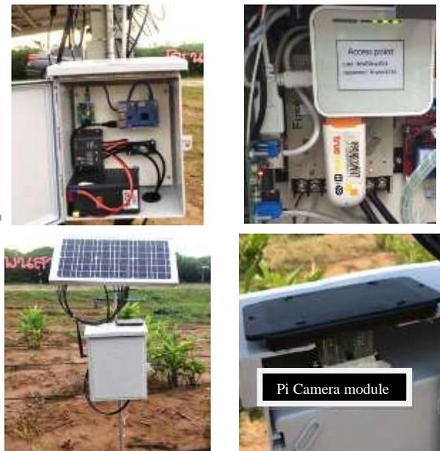
Figure 5: The compression and decompression node installation at SUT farm
