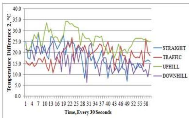
Figure 6: Temperature Diff (Exhaust) Vs Time
