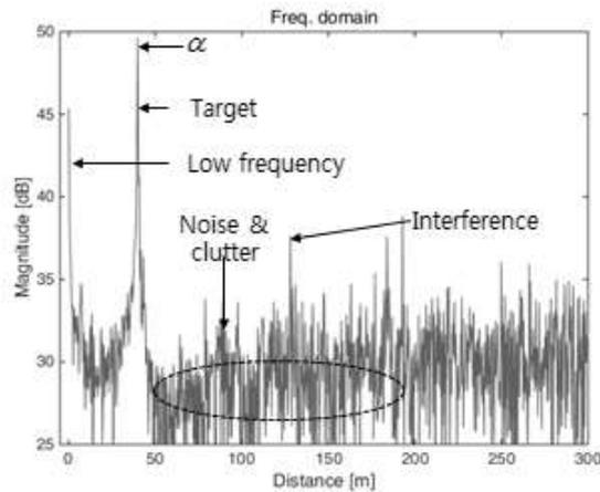
Figure 1: RCS configuration: received signal in the frequency domain.
