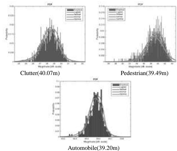
Figure 5: Probability distribution for the measured RCS of targets and clutter (near 40m)
