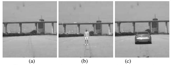
Figure 2: Distance 20m (a) clutter, (b) pedestrian, (c) automobile
