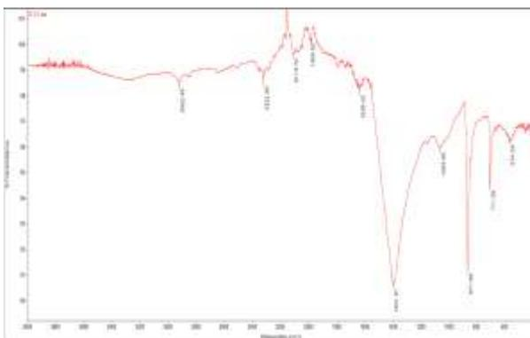
**Fig. 7:** FTIR spectrum of recovered duck eggshell calcium carbonate
