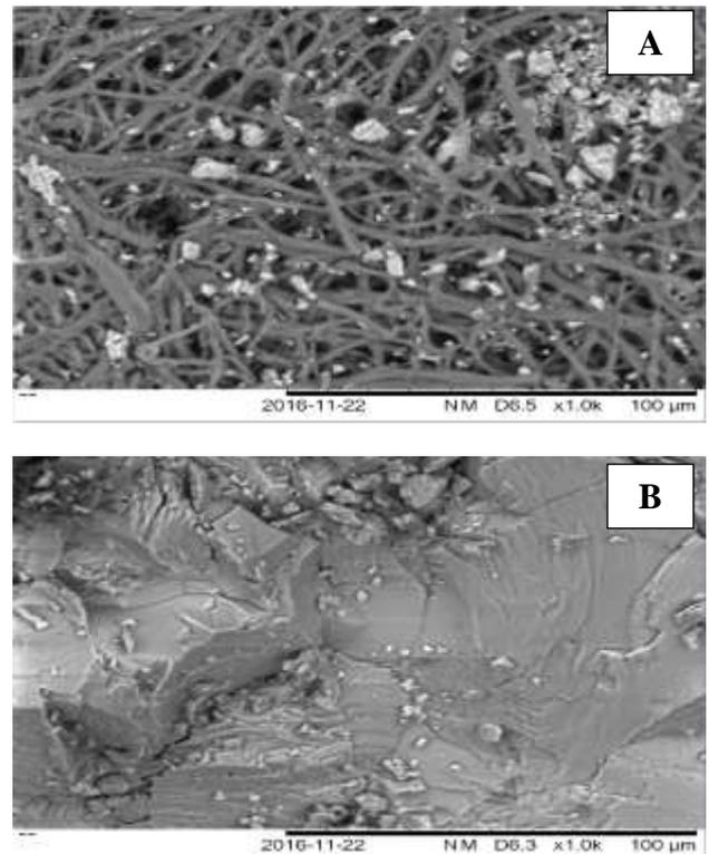
Fig. 5: SEM images of duck eggshell at magnification of 1000x (A) Before DAF and (B) After DAF
