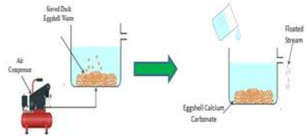
Fig. 1: Sketch of DAFT for duck-egg shell calcium carbonate recovery
