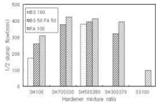
**Figure 3:** 1/2 slump test
