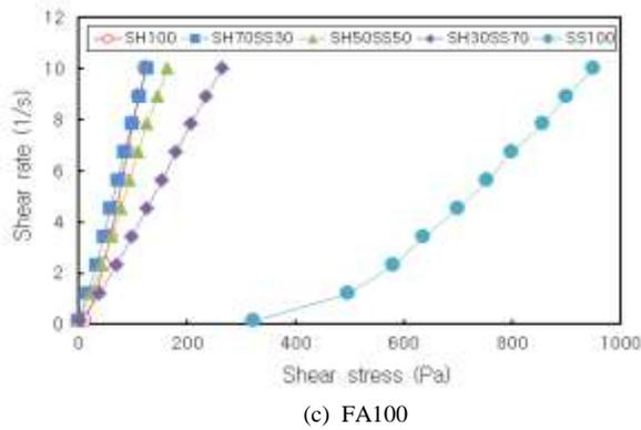
Figure 4: Consistency curve of alkali-activated mortar
