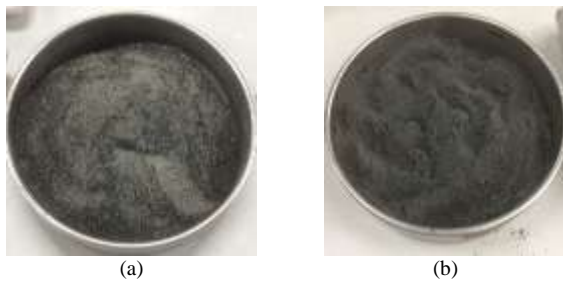
Figure 1: (a) Unground POFA and (b) Ground POFA
