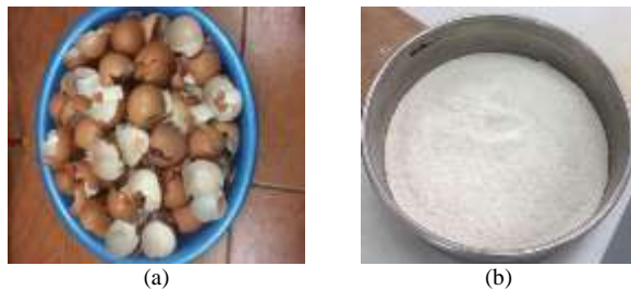
Figure 2: (a) Egg shells and (b) egg shell powder after ground
