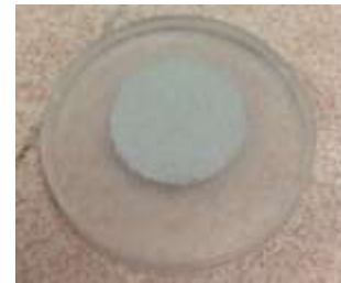
Figure 3: Mortar sample of mix C80GP16E4 for XRD testing
